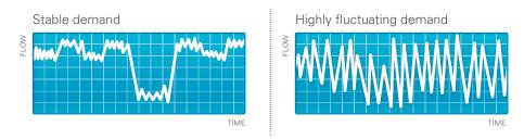
The ZH 350<sup>+</sup> handles air demand fluctuations more effectively than turbo technology could do up to now. Its fast transitions between load and unload operation eliminate the need for expensive blow-down of compressed air in times of low air demand.
