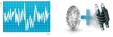
The combination of turbo and screw brings the energy bill further down in larger compressor rooms. While the Variable Speed Drive (VSD) screw accommodates the large fluctuations, the turbo efficiently takes care of the base flow requirements.
